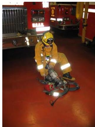
Always return SCBA to the ready to go position, Make sure that bottle is full and regulator is placed in the protective dust cup.
