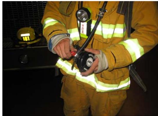
Push inward and close cylinder valve. Bleed residual pressure using the purge valve.
