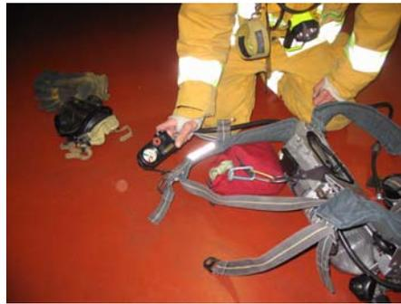
Push in and turn cylinder valve counter-clockwise, fully open. Compare pressure on remote gauge to pressure on cylinder.
